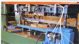
Lubricating the "trouble" stations in a Transfer Die.
