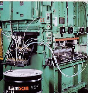
PresSpray II Mounted on a Bracket w/Optional PowerPump Attached
