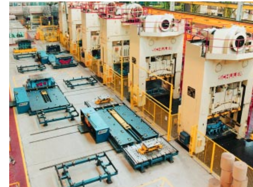
Three dual-station die carts and 12 die racks are integrated with a robotically-loaded 6-press tandem line to economically achieve an 80% reduction in changeover time at LDV (Birmingham, UK) for Just-in-Time operations. Over 140 tandem press lines around the world have been equipped by Atlas.
