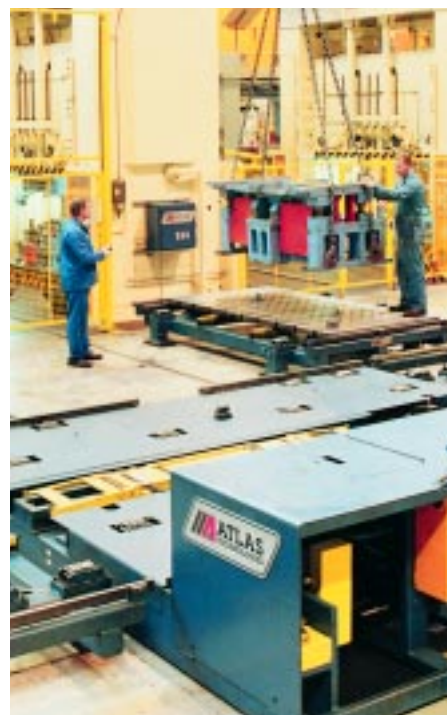
Dies are pre-staged prior to changeover. Attaching every die to a common-sized subplate provides uniformity for die positioning in the press and all die movement on carts and racks.
