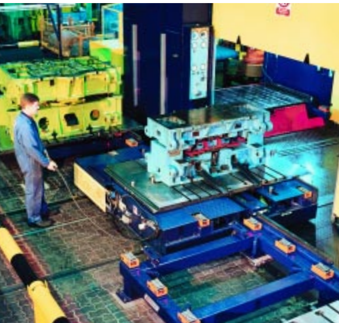
A single cart and two racks can serve two stand-alone or tandem line presses.
