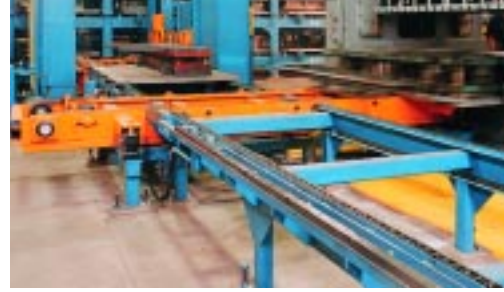
Die change in progress on a 3-station T-Table at John Deere's Ottumwa, Iowa facility.
