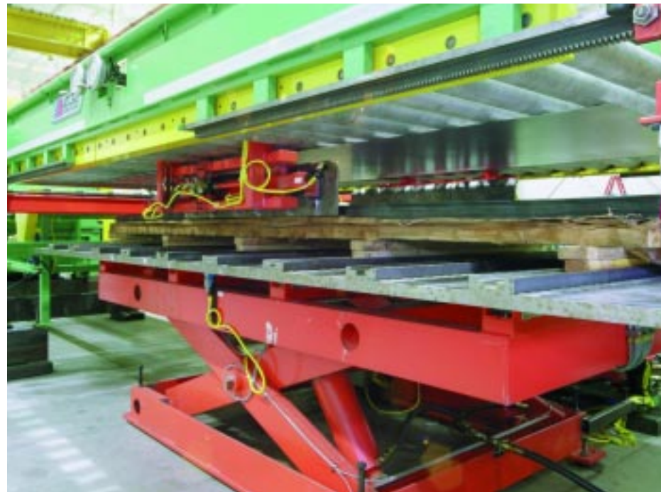
Blank stacker drops blanks to wood dunnage which is supported by a lift table that minimizes drop distance.
