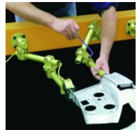
FLEX articulated Finger Tooling lets you adjust one axis at a time, reducing trial-and-error setup time on your transfer press.
