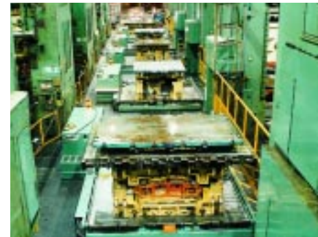
Automotive body panel stampers are achieving completely automatic, "one-button" die changeover with Atlas systems. Here, between-press automation automatically moves out of the way as seven die carts simultaneously move in and exchange the dies.
