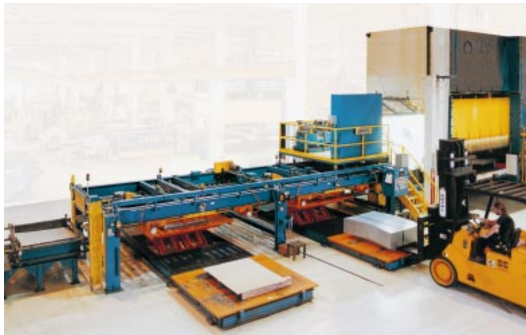
Double-station blank stacker alternates between the two stations, allowing continuous blanking and stacking, with no interruptions for stack removal. Full pallets move to either side of the stacker via conveyor. A reject station is at end of stacker (at left).
